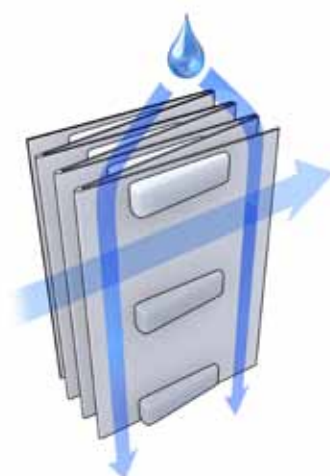
Open hot melt separators allows water to drain
